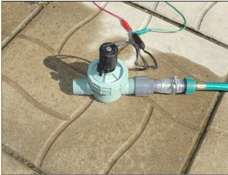
An Orbit sprinkler valve connected to a garden hose for testing purposes. The other side (water output) is just left open.
