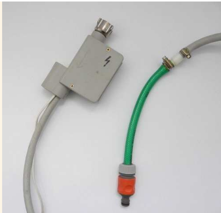
A magnetic water valve taken from an old dish washer. It connects directly to the water tap and you can attach a garden hose to it.
