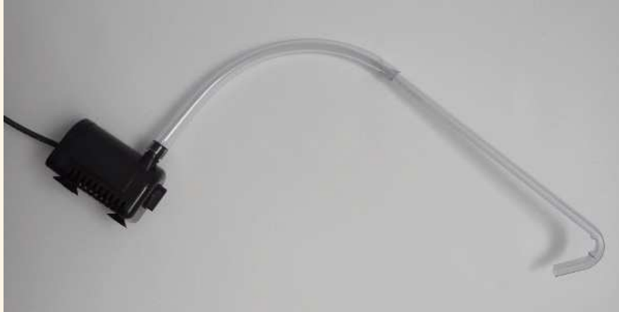
The submersible water pump from siliconsolar.com I attached a short hard plastic tube to the hose and I bended it like a little hook at the end.
