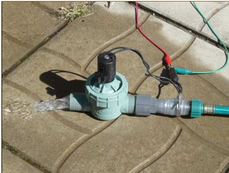
Power-on and water flows. The sprinkler valve works. We can now install it properly.
