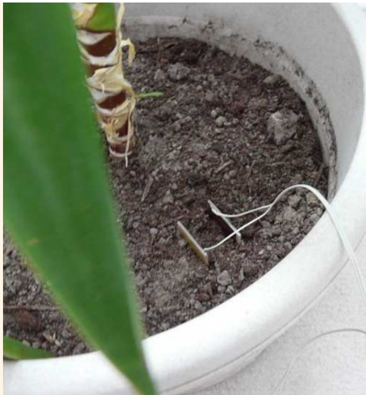
The capacitive humidity sensor in action
