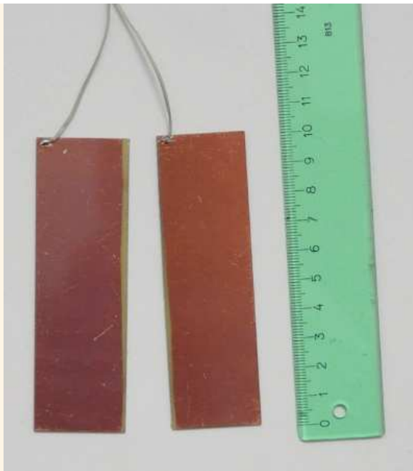
Two pieces of PCB insulated and painted with clear coat.
