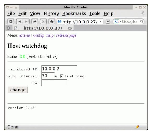
The watchdog is configurable via its own web-pages. You just point your web browser to it and you can see the state of the system, how often it had to be reset, if the watchdog is active or passive etc.... You can also configure if ping shall be sent from the watchdog or if the system will ping the watchdog.
