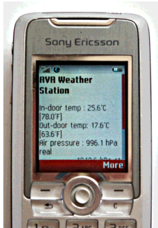
The Ethernet Weather Station as seen from a Mobile Phone
