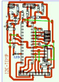
I used the orange colored layer for drawing. Somehow the other layers would not generate any output when printing. The problem is that the orange colored layer is acutally on the side of the board where the parts are. If you write text in this layer then it has to be mirrord when you print it on the physical board. Therefore I made the basic layout with pcb and all the rest with gimp.
