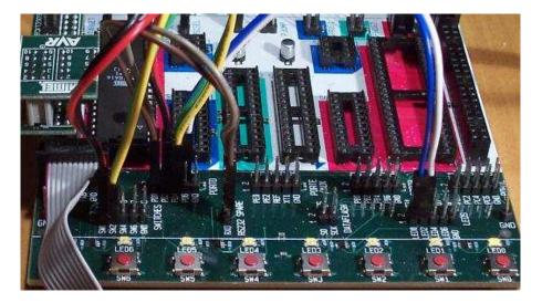
Figure 7: Wiring of the STK500
