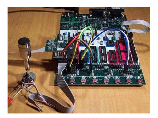
Figure 6: Setup of the STK500
