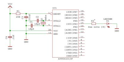
Figure 5: Schematic of circuit for demo project
