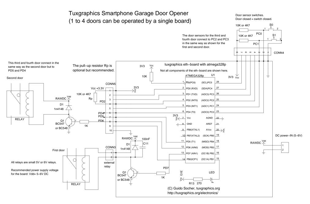
Note: different tuxgraphics ethernet boards have different connector layouts. Important are only the pin names at the microcontroller such as PC0, PD6,...GND, Vcc3.3V...
