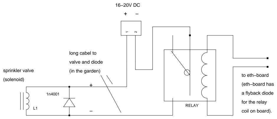
Flyback diode to block high voltages induced by the sprinkler valve coil when the relay opens
